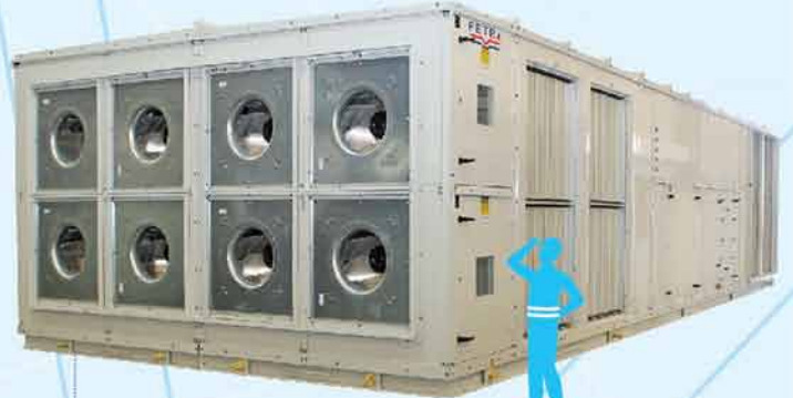
▶ Air Cooled Rooftop Package Unit with VSD Scroll Compressors and EC Supply and Return Fans 180 T.R. (630 kW) 70,000CFM (33,000 l/s)
